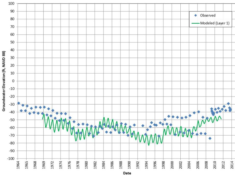
Figure 11h: Groundwater Elevation, Calibration Well 201
