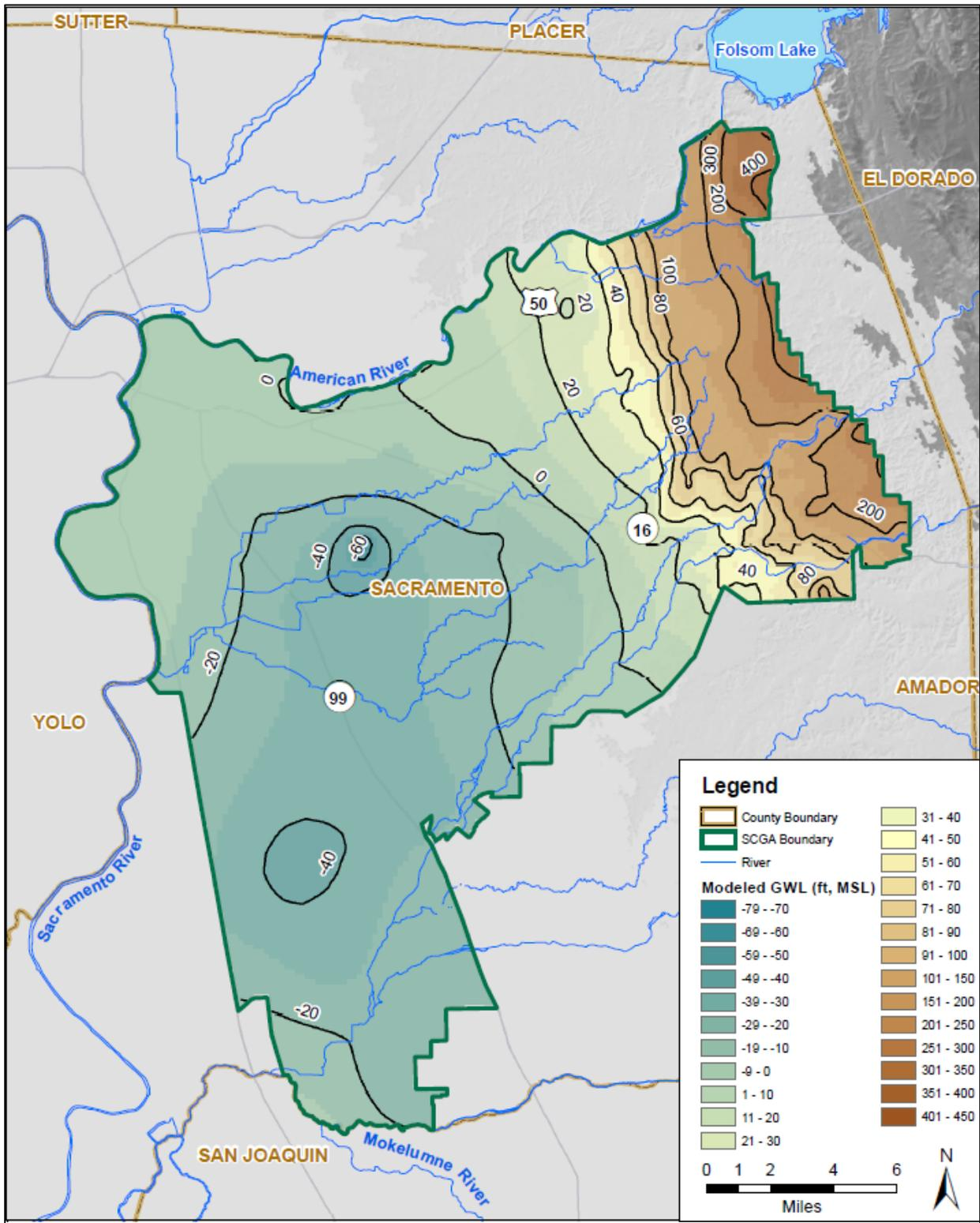
Figure 10: Groundwater Elevation Contour Map at the End of Simulation – 2030 Baseline Model
