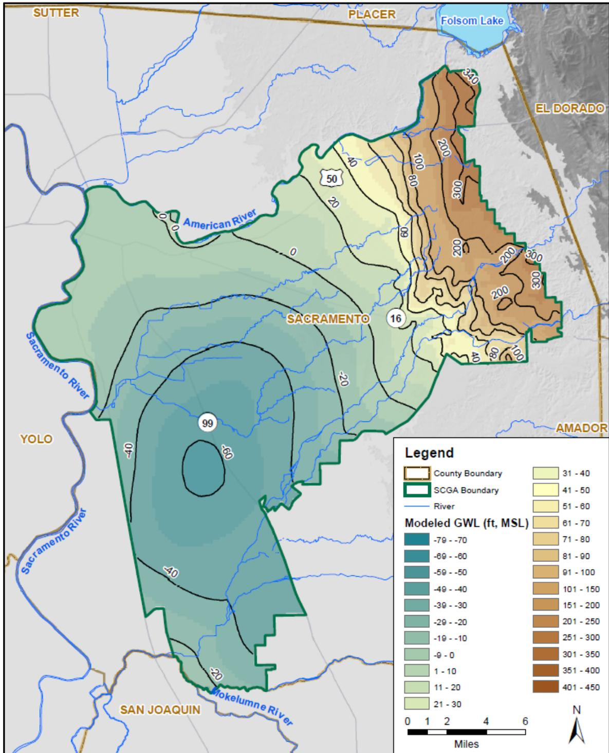
Figure 13: Groundwater Elevation Contour Map at the End of Simulation –
