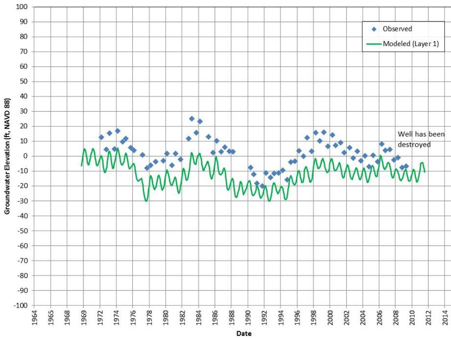
Figure 11f: Groundwater Elevation, Calibration Well 122
