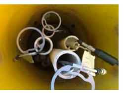
Nested monitoring wells (multiple casings in a single borehole)
